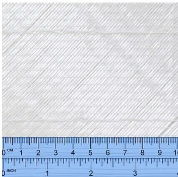
**Pros:** Strength in Two Directions: With fibres running at  $0^\circ$  and  $90^\circ$  or  $+ - 45$  degrees, biaxial weaves offer excellent strength in two main directions.
