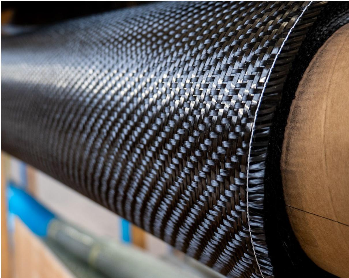
**Pros:** Excellent strength-to-weight ratio with sleek aesthetics. It has both high stiffness and strength compared to glass fibres of similar weight per square metre, so perfect for much lighter weight panels with less flex. It is Corrosion resistant and has good X-ray transparency, Low CTE (Coefficient of Thermal Expansion), Chemical resistivity, Thermal and electrical conductivity.
