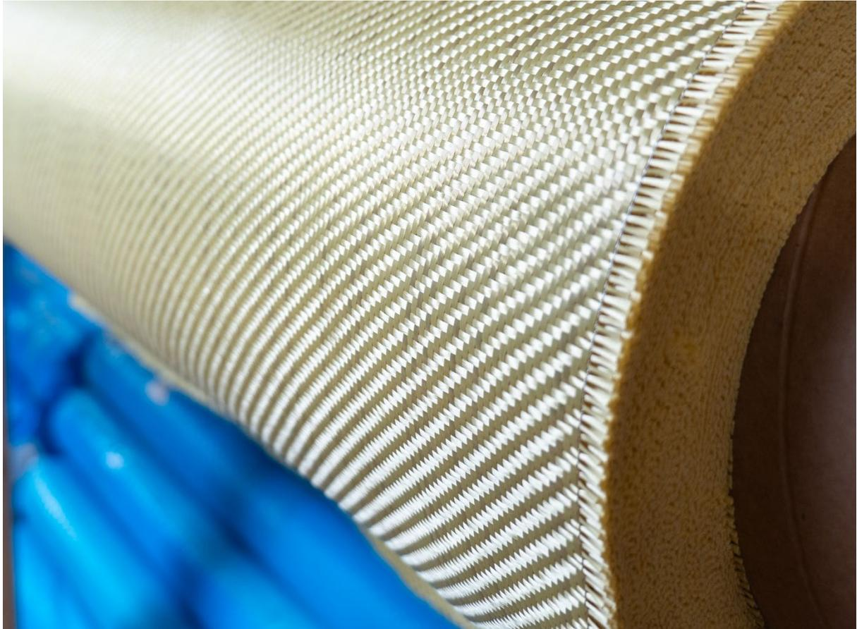
**Pros:** Great impact resistance, superior tensile strength, lightweight. The tensile strength of Kevlar® is over eight times greater than that of steel of equal weight. It also withstands the extremes of temperature as well as the effects of salt water and other natural occurring chemicals.
