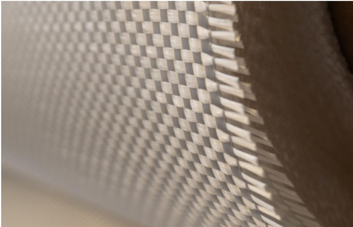
**Pros:** High Impact Resistance: Diolen offers excellent resistance to impact, making it suitable for products requiring high durability. It is also more economically priced than that of Kevlar® if you want high impact resistance without abrasion resistance.
