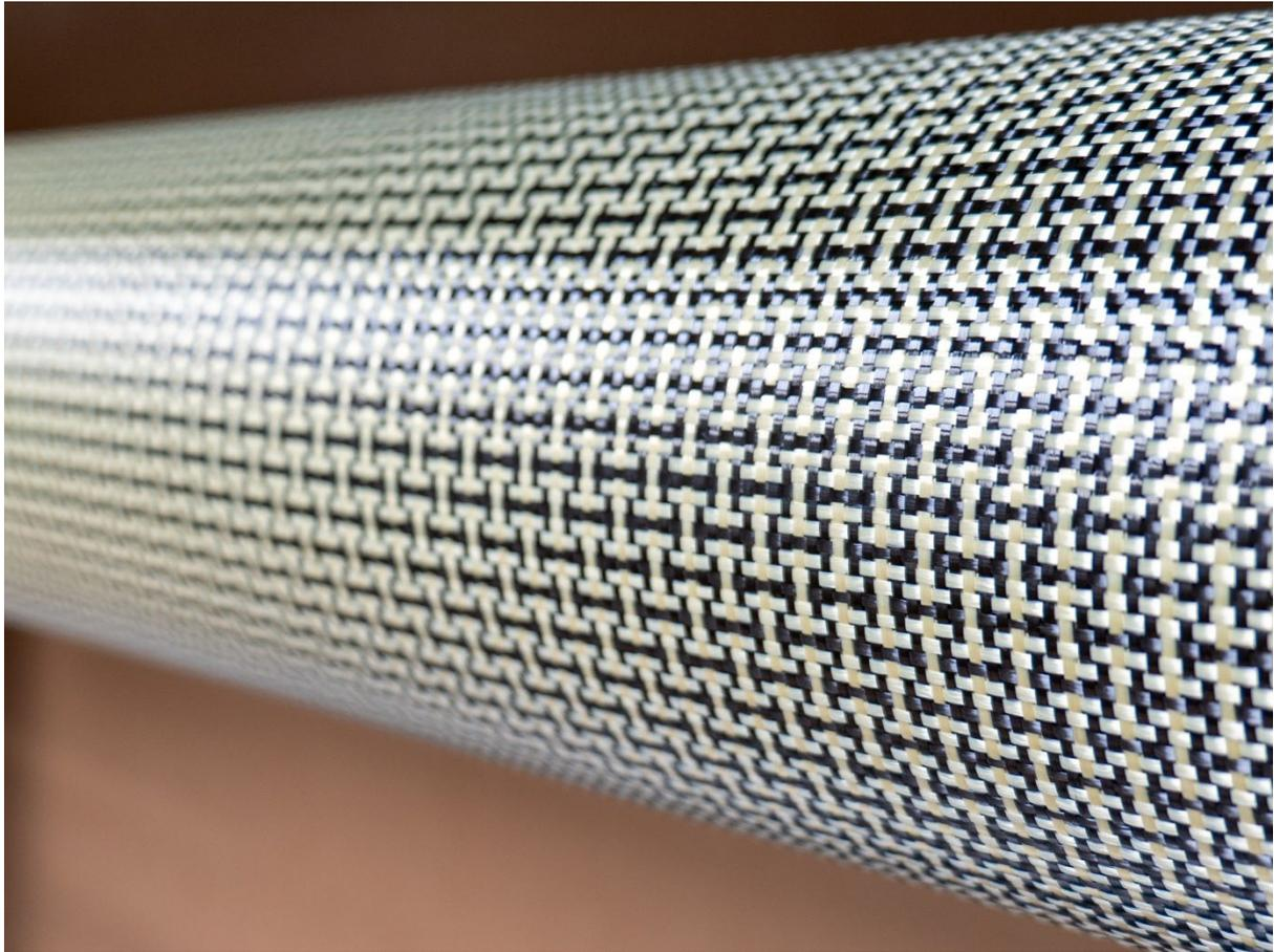
**Pros:** Combined Properties, Hybrid fabrics, like carbon-Kevlar® mixes, combine the benefits of different materials, offering both strength and impact resistance.
