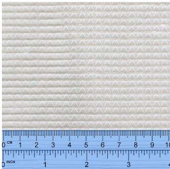
**Pros:** Multiaxial Strength: Combines fibres in four directions, offering excellent strength and stiffness in various orientations.
