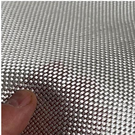
**Pros:** Stability: This traditional over-and-under weaving pattern offers stability and maintains its shape well.
